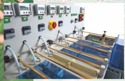
as a general-purpose electroplating plant, for the chemical or electrochemical treatment of metals in vertical technology. In consultation with the customers requirements the desired through-hole plating system is constructed.
