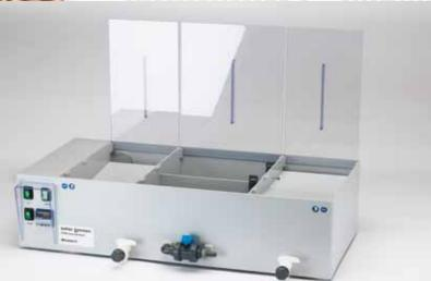
ping, etching and rinsing (optional stripping) in one unit and enable the production of highquality PCB structures of 50-100 microns. The units are designed for prototypes and small series of up to a suitable plate size of 500 x 600 mm.
