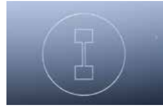
An example of milling lines on a silicon wafer
