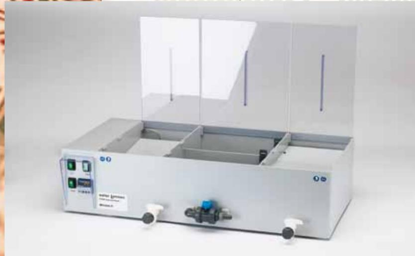
The laboratory bench systems of series MINISTAR and the floor-mounted units of the series ETCHING CENTER V are used for developing, etching and rinsing in foam-etching process and continuous development process. They are ideal for the processing of small printed circuit boards and etched plates in laboratories, schools and institutions to create professional sample sheets and prototypes.
